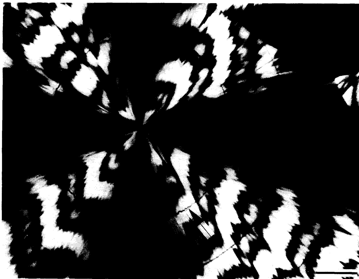
Figure 1 Optical micrograph (crossed polarizers) of a PHB spherulite grown at 95°C showing black circumferential features (arrowed). Scale bar 100 \mu\text{m}
